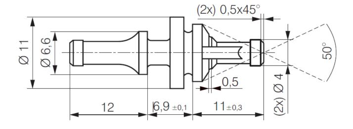
Rubber anti-vibration mounts for fans with a hole diameter of  $4.3 \pm 0.2$  mm and flange thickness of 3 to 5.5 mm. For a carrier plate with a hole diameter of  $6.5 \pm 0.15$  mm and plate thickness of 1 to 2 mm.
